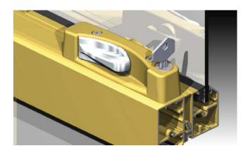
We have designed a completely new lock for this window. Roll the chrome handle over  $180^\circ$  to lock/unlock. The bold 30mm thick sashes have been designed to accept a variety of glass thicknesses from 4mm to 20mm thick.
