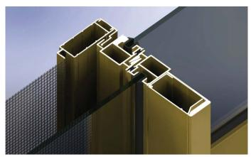
A key feature with Series 541 is the clean fly door installation. The screen doors have snap-on interlock that nests into the interlock on the glass door. This removes unsightly visible rivets or screws that would occur with plant-on interlocks. This illustration shows the meeting stile span-in closer feature.
