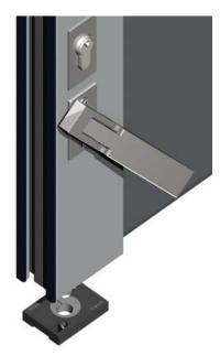
The picture above shows the optional ICON™ bolt activator (only available in 316 stainless steel). Turn the lever 90° to retract top and bottom bolts. This picture also shows another feature with Series 548 − The adjustable bolt keeper. This keeper allows us to tighten or loosen the panel to frame joint.
