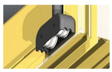
Bottom rollers are more reliable for residential projects as top hung panels can run into problems if the head lintel sags.
