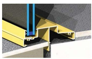
Fixed sidelights on Series 549 have been designed to match the hinged door frame and again look like a bold timber frame. Both doors and sidelights will accept glass up to 20mm thick.
