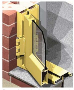
This external opening door sill is splayed to the outside to ensure all surface water drains out of the system. This detail also shows an optional custom parliamentary hinge that allows door to swing right back against the wall.
