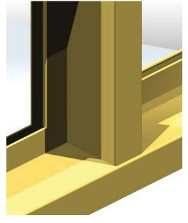
This illustration highlights one of the features on Series 602 – The 2mm soft radius on the inner edge. We recess the mullions 2mm to clear the perimeter frame edge radius. This removes the chance of unsightly edge joints. This treatment is similar to what is done with timber windows.
