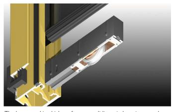
The key to making high performance sliding windows is to use large diameter high performance wheels. We use sliding door wheels in Series 602 and when the panels are double glazed or extra heavy we use double bogey wheels.
