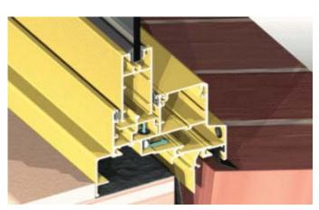
Sill fitted with anti blow back ball valve. This allows water to escape while controlling the air flow.
