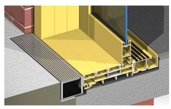
The above illustration shows the four track XXXF flat sill with recessed sump on the outside and Centor S1 roller screen on the inside – Completely flat sill design feature.
